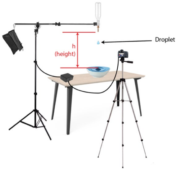
Figure 9. Sketch of how this device was tested.
