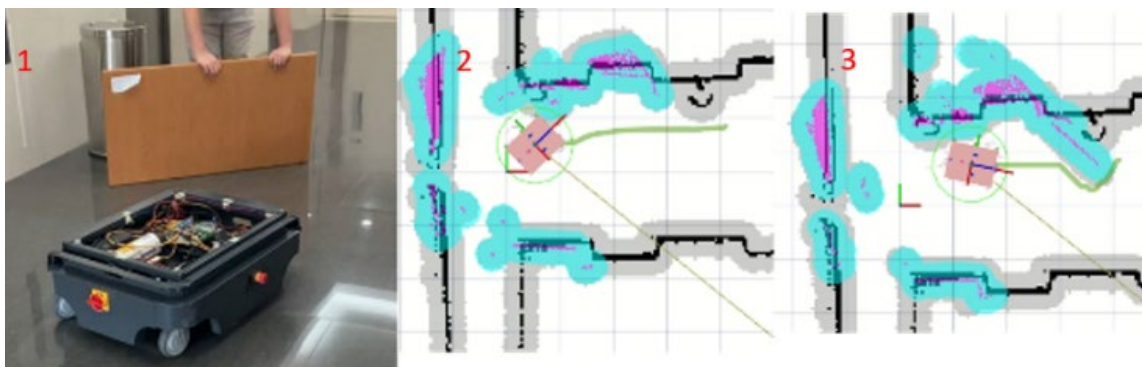
Figure 7. Navigation and obstacle avoidance test, (1) set up; (2) initial; (3) final state.
