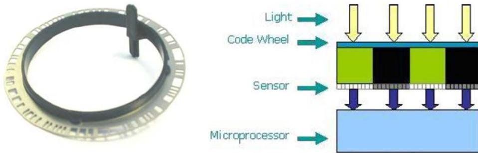
Figure 6. Steering sensor made by Methode Electronics [11]
