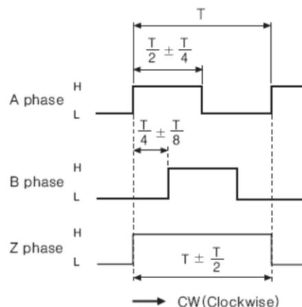
Figure 8. The output of the wave A, B, and Z [13]
