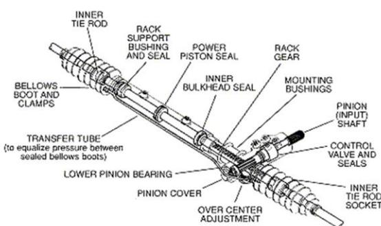
Figure 2. Rack and pinion-type steering transmission [2]
