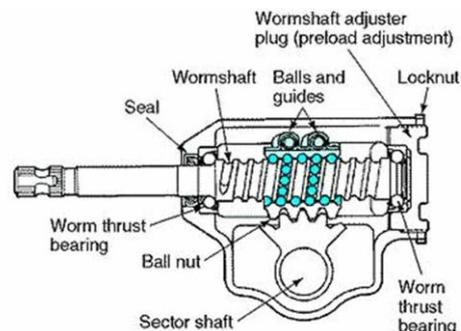
Figure 3. Screw and sector-type steering transmission [3]
