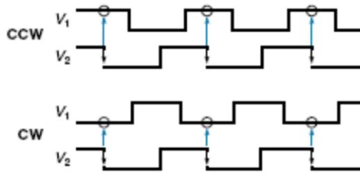
Figure 9. Direction determination through V1 and V2 processing [3]
