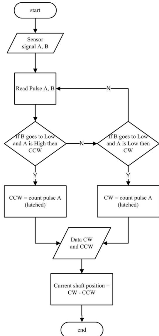
Figure 10. The flowchart process counting of steering shaft position
