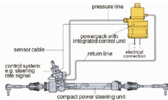
Figure 4. The scheme of electro-hydraulic power steering (EHPS) [5]
