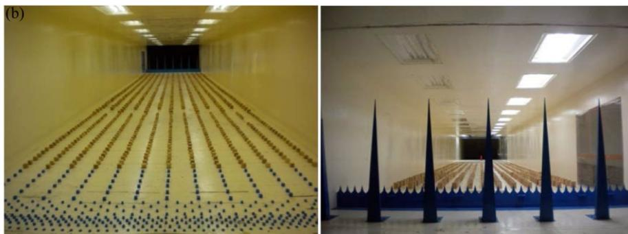
Figure 3. (a) Wind tunnel at CKP wind solutions, South Korea; (b) Roughness block of terrain B in wind tunnel experiment
