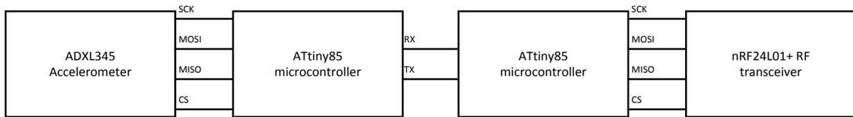
Figure 3. Block diagram of the transmitter module
