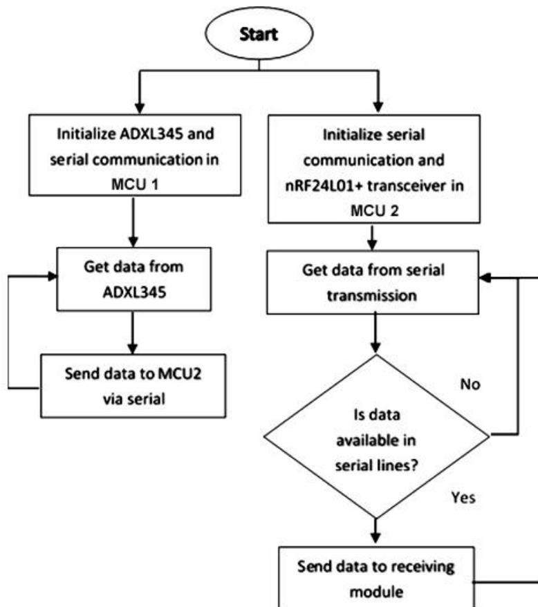
Figure 4. Flow chart for the transmitter module hardware program
