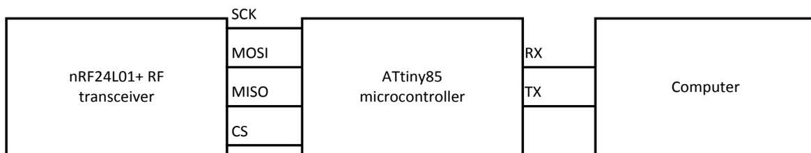
Figure 5. Block diagram of the receiver module
