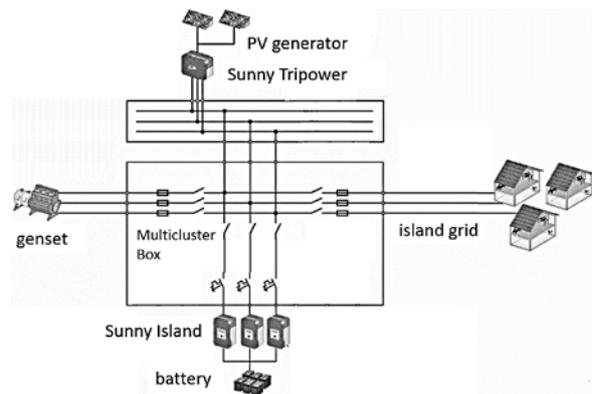
Figure 5. System structure
