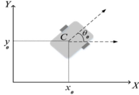
Figure 1. Wheeled mobile robot motion on the X-Y plane
