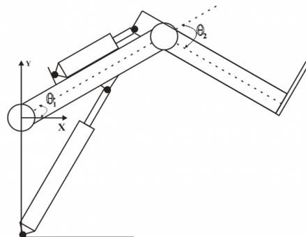
Figure 5. Model of rehabilitation lower limb actuator
