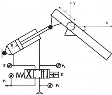
Figure 6. Model of control at each joint
