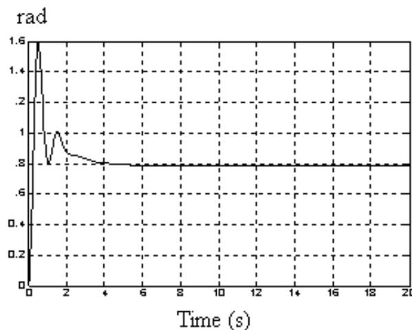
Figure 11. Angle response of joint 1
