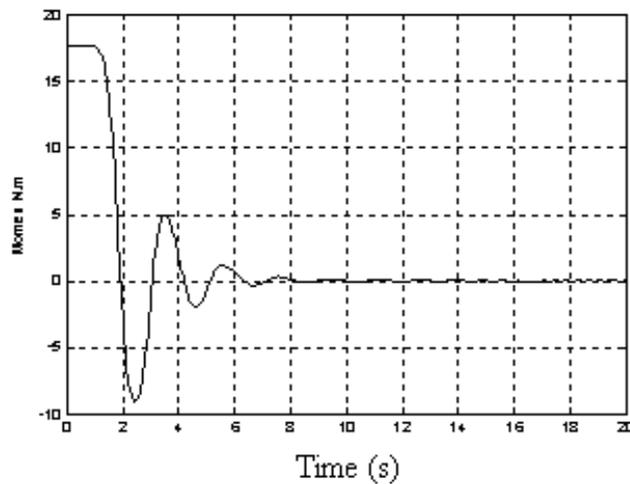
Figure 10. Torque response of joint 2
