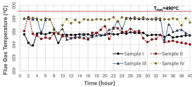
Figure 16. Profile of flue gas temperature
