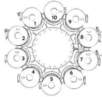
Figure 12. Combustor chambers [6]
