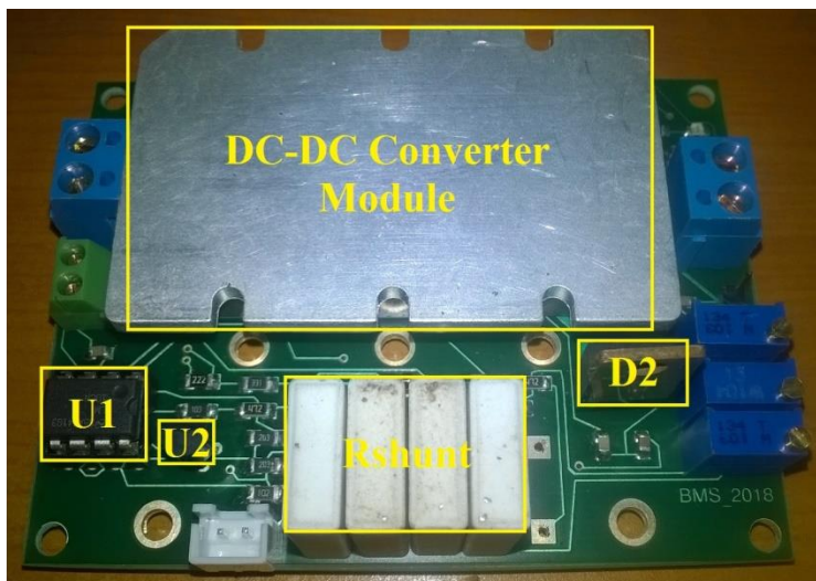
Figure 4. LiFePO 4 battery charger prototype
