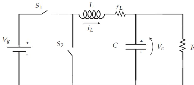
Figure 1. The schematic of a DC-DC buck converter
