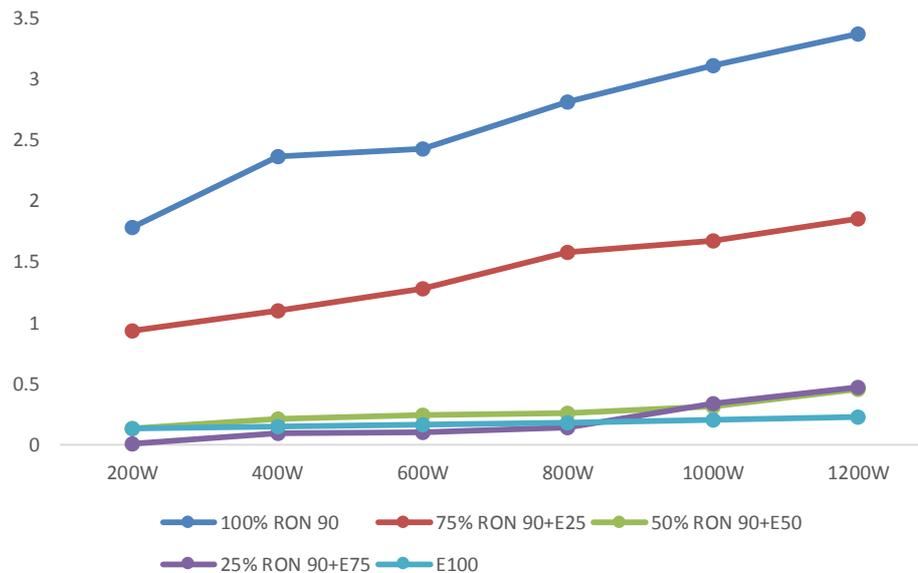
Figure 1. Comparison results of CO exhaust emission (in vol%)
