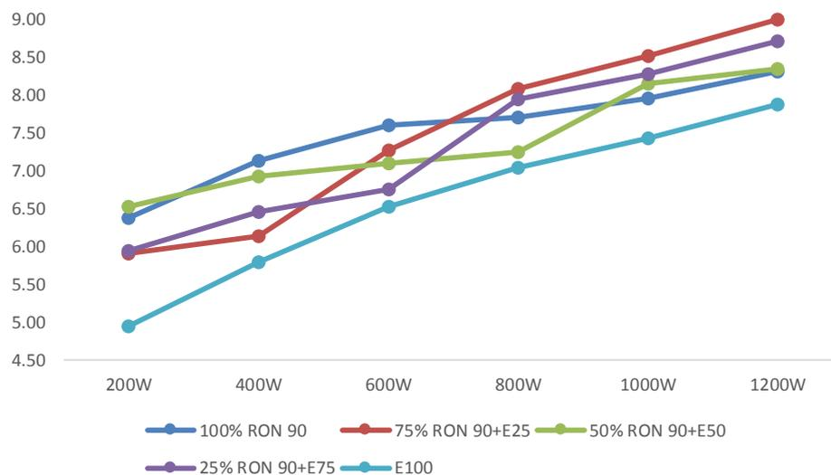
Figure 2. Comparison results of CO<sub>2</sub> exhaust emission (in vol%)
