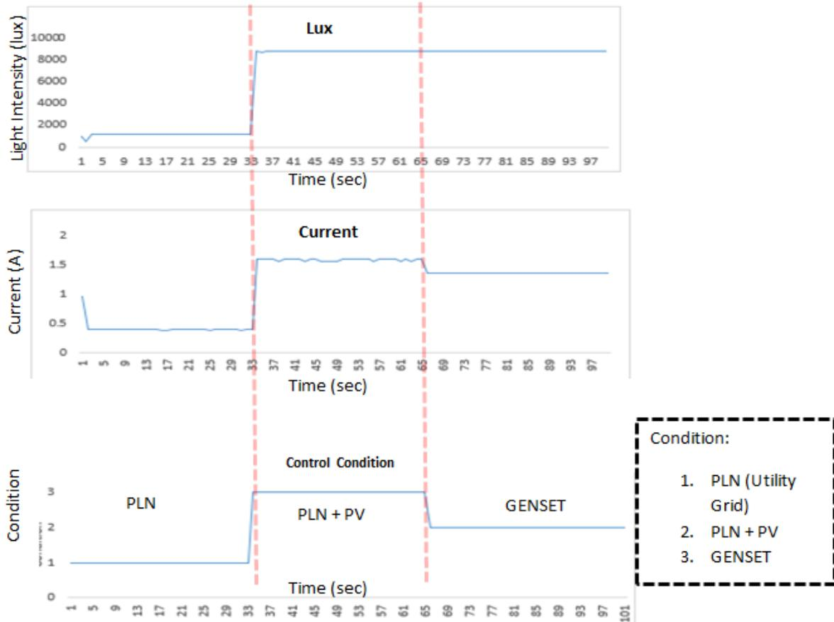
Figure 13. Testing of smart grid system using LaC
