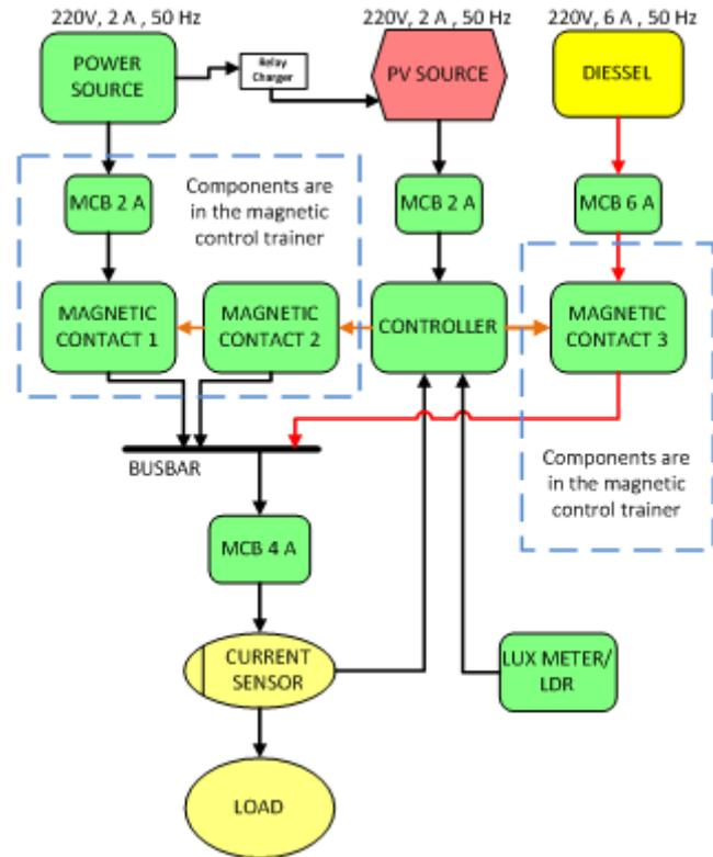
Figure 2. Smart grid lab-scale construction
