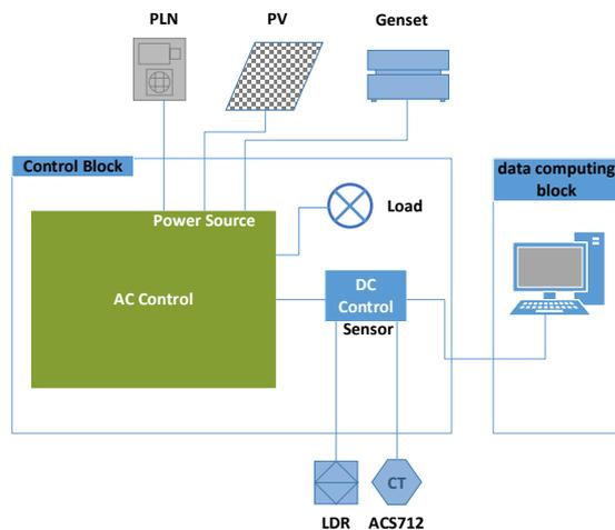
Figure 4. Design of lab-scale smart grid system
