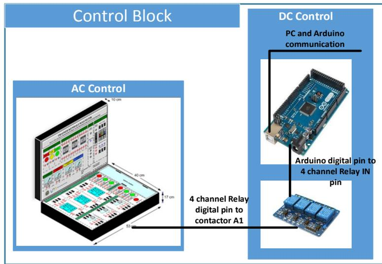
Figure 5. Lab-scale smart grid system full block design
