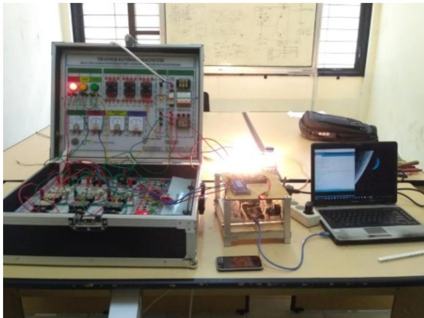
Figure 12. Smart grid system testing using LaC
