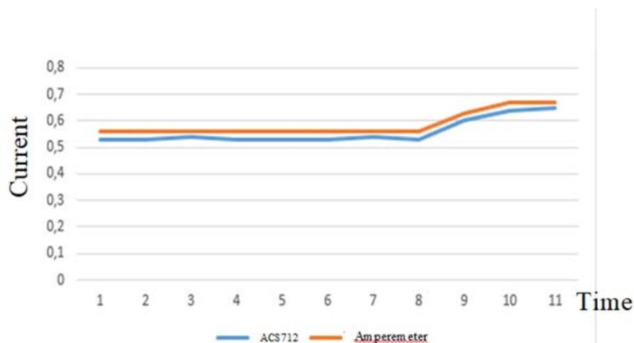
Figure 10. Comparison of ACS712 and amperemeter measurements
