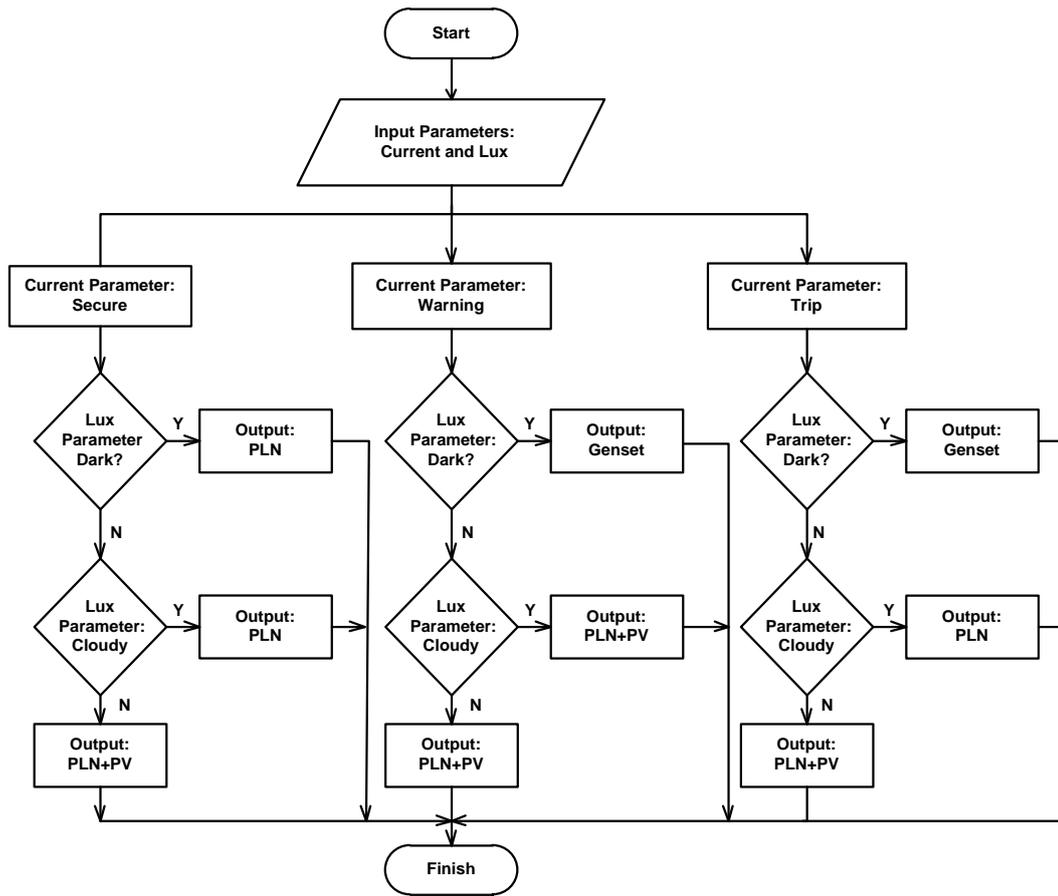
Figure 1. Lab-scale smart grid system flowchart
