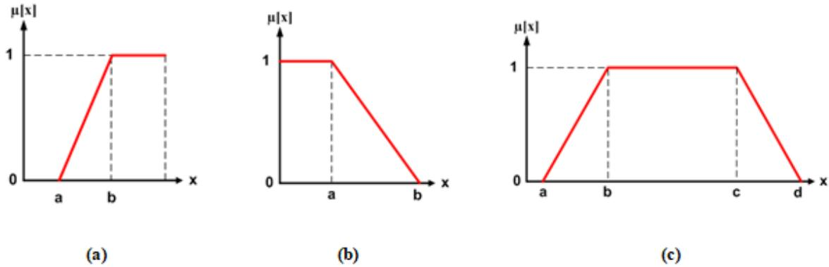
Figure 8. Membership function: (a) Linear up; (b) Linear down; and (c) Trapezoid
