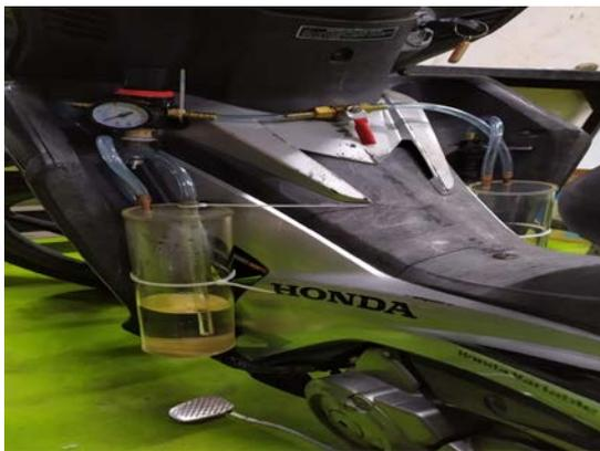
Figure 6. Cooling cylinders and gas reservoirs
