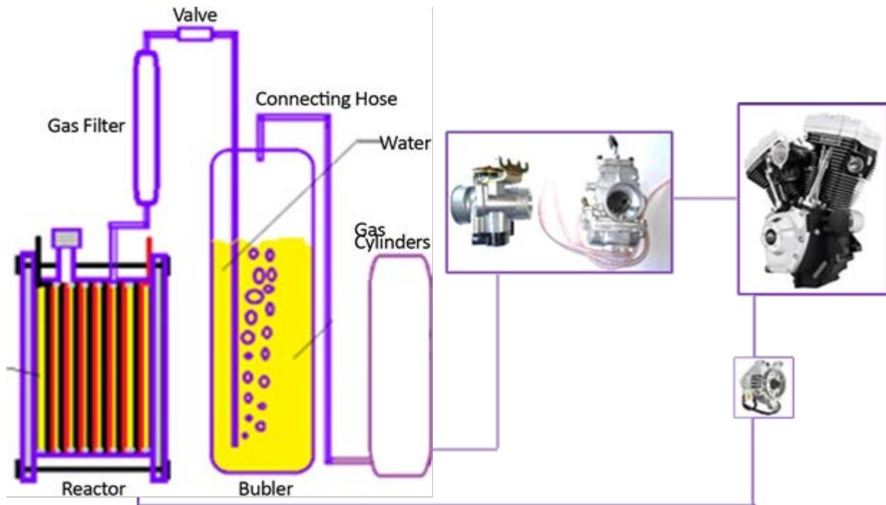
Figure 3. Electrolysis process schematic
