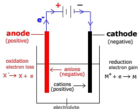
Figure 1. Water electrolysis circuit [18]
