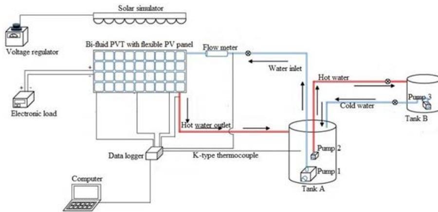
Figure 2. Schematic of experimental setup for PV with cooling system
