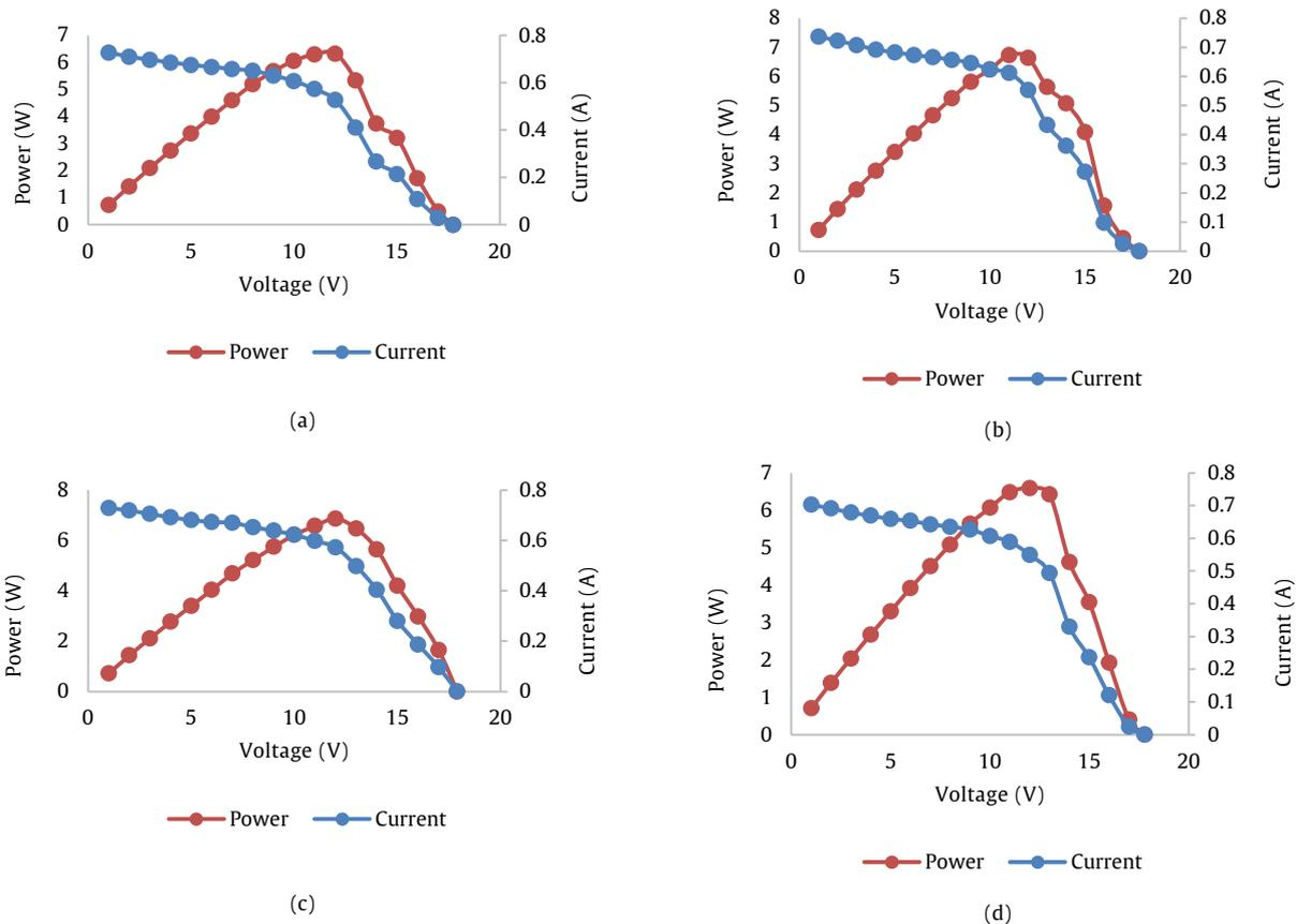
Figure 4. I–V–P curve for the average test conducted at: (a) 0.04 kg/s of air mass flow rate with fixed rate of water mass flow; (b) 0.06 kg/s of air mass flow rate with fixed rate of water mass flow; (c) at 0.08 kg/s of air mass flow rate with fixed rate of water mass flow; (d) at 0.1 kg/s of air mass flow rate with fixed rate of water mass flow
