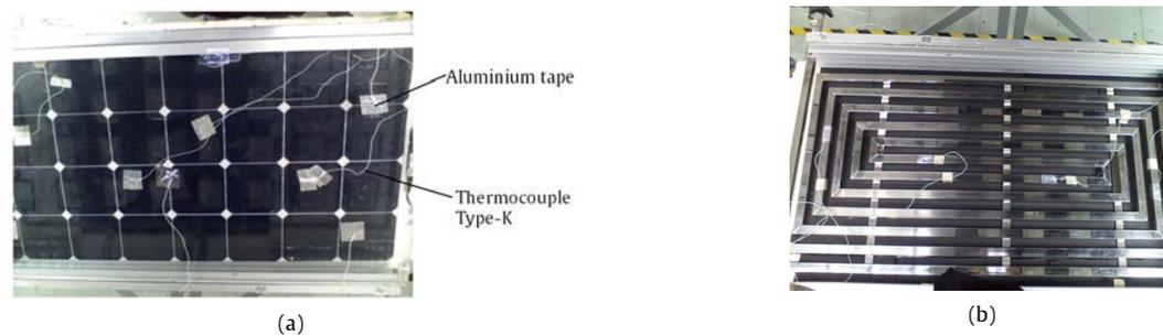
Figure 1. (a) Flexible photovoltaic panel (Table 1); (b) integrated with spiral absorber (the water flow channel)
