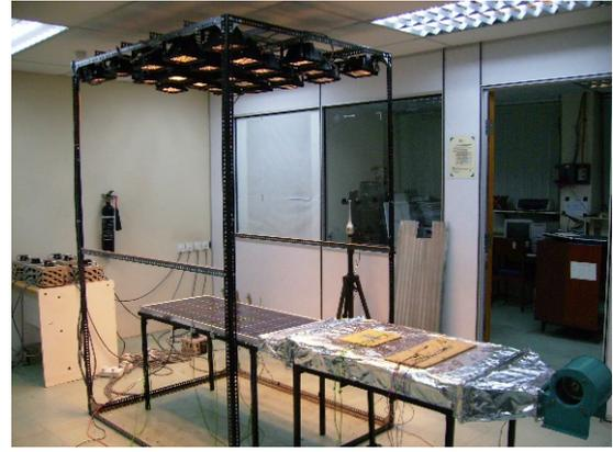
Figure 2. Photograph of PVT air collector under solar simulator
