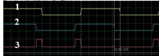
Figure 12. Wave input and output IC 74LS86 at phase angle 27°. (1) Current-phase currents (2) Square wave phase voltage; (3) Square wave difference of phase current and voltage
