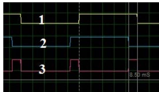
Figure 13. Square wave as an indicator of phase difference at moment 27°. (1) Current phase input waves to IC 74LS86; (2) Wave input of phase voltage to IC 74LS86; (3) Wave output of IC 74LS86 as phase angle in time
