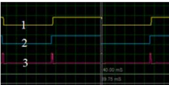
Figure 27. Wave input and output IC 74LS86 at phase angle  $4.5^\circ$ . (1) Current-phase currents; (2) Square wave phase voltage; (3) Square wave difference of phase current and voltage
