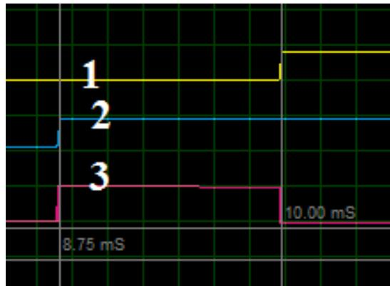
Figure 16. Square wave as an indicator of phase difference at a different phase of 22.5°. (1) Current phase input waves to IC 74LS86; (2) Wave input of phase voltage to IC 74LS86; (3) Wave output of IC 74LS86 as phase angle in time
