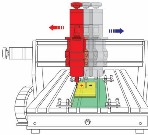
Figure 4. Machine path on making markings
