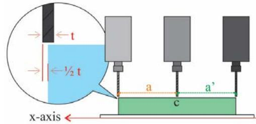
Figure 5. Guidance on making the two markings on x-axis
