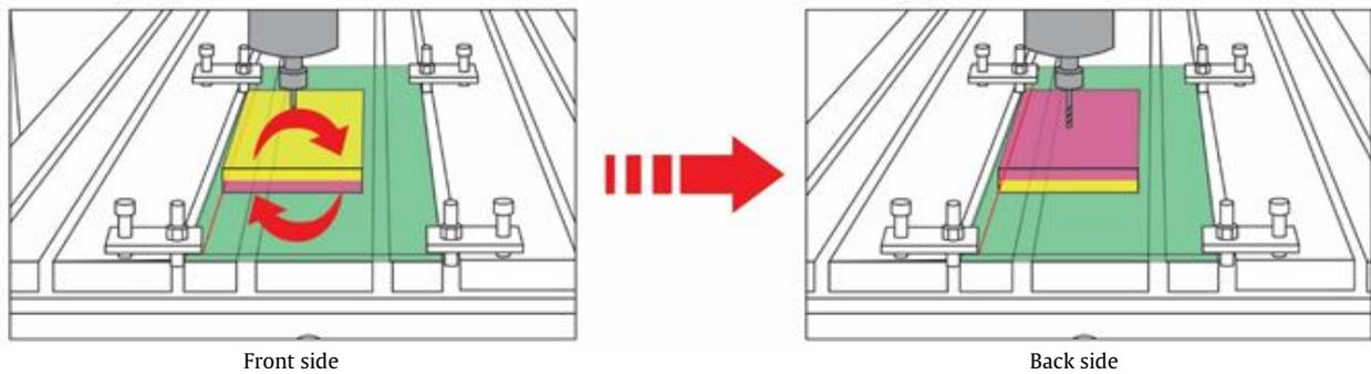
Figure 7. Flipping material to do back-side machining
