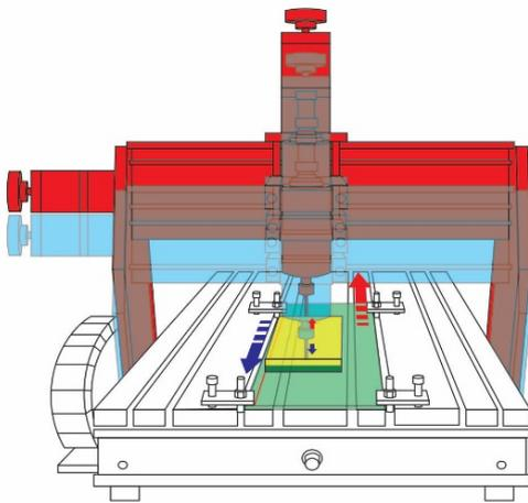
Figure 9. Machine path on making markings
