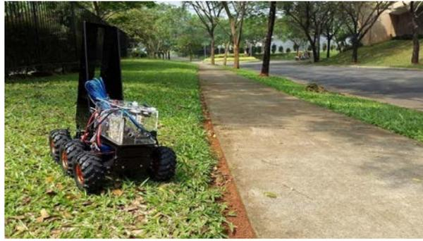
Figure 18. The robot falls from the road because of an inaccurate road angle
