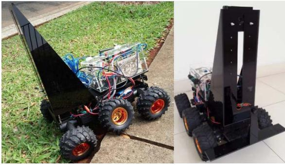
Figure 2. Fully constructed autonomous mobile robot for outdoor navigation
