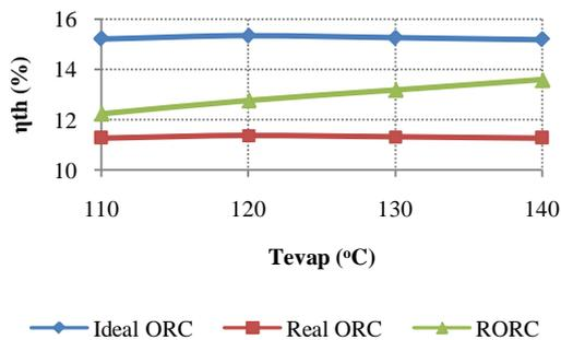
Figure 11. Thermal efficiency at varying evaporating temperature
