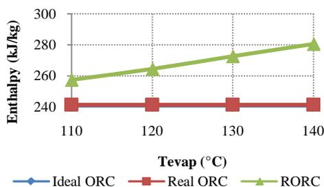
Figure 7. Enthalpy entering evaporator at varying evaporating temperature
