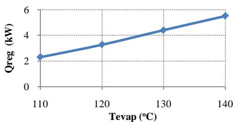
Figure 6. Regenerator capacity at varying evaporating temperature
