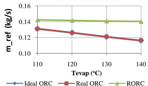
Figure 8. Refrigerant mass flowrate at varying evaporating temperature
