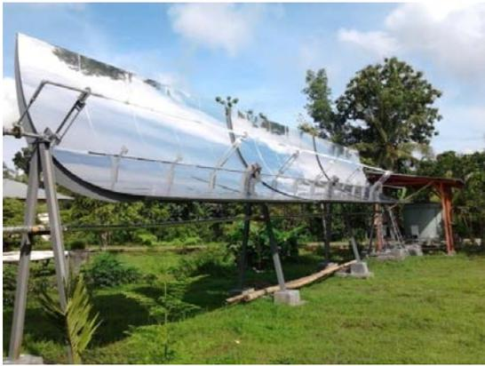
Figure 2. Parabolic trough solar collector (PTSC)
