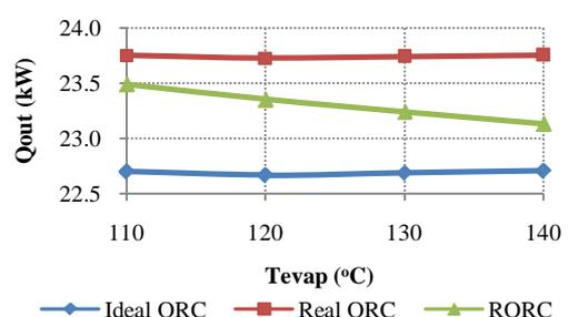
Figure 9. Heat output at varying evaporating temperature
