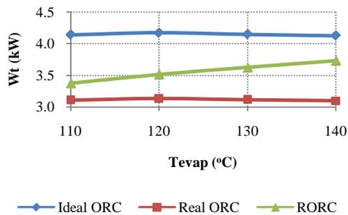
Figure 10. Turbine power at varying evaporating temperature
