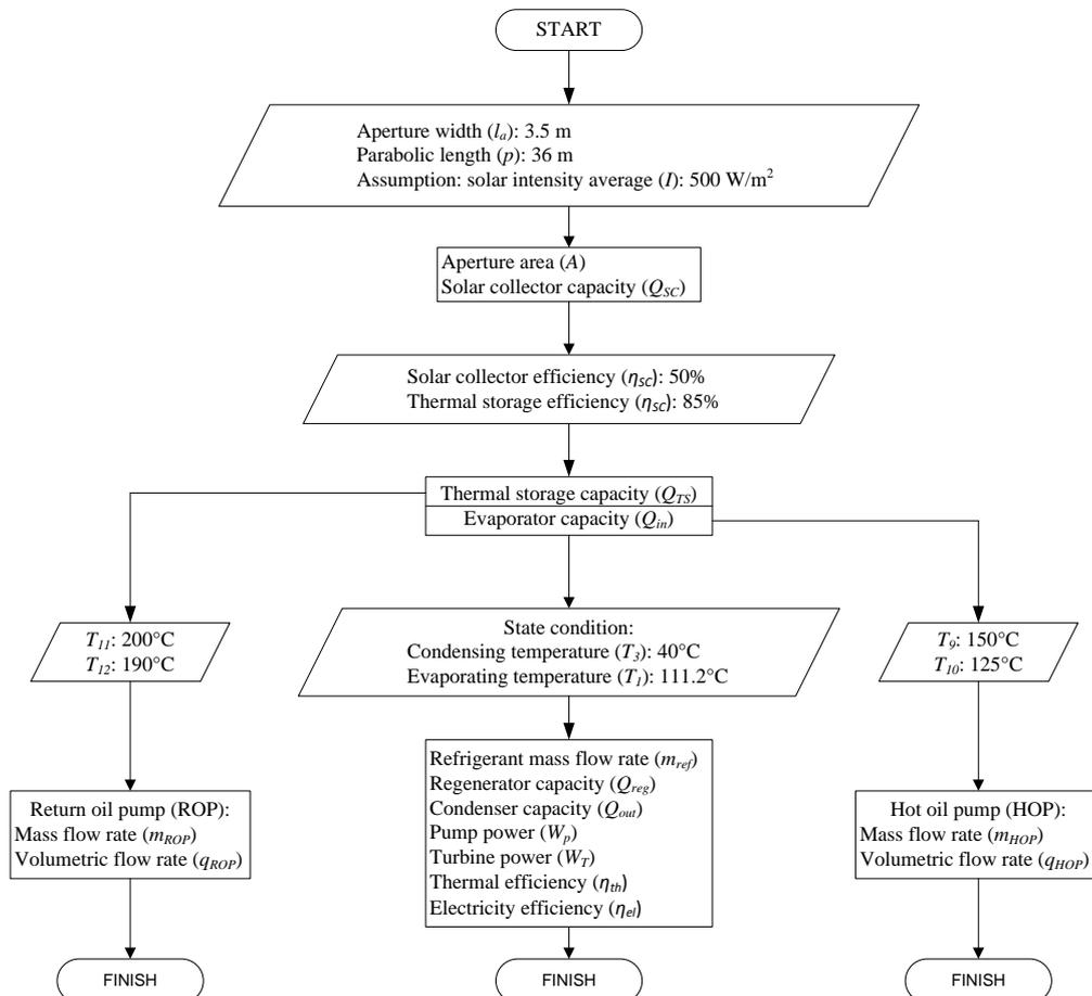
Figure 3. Flow diagram design optimization of solar thermal power using RORC
