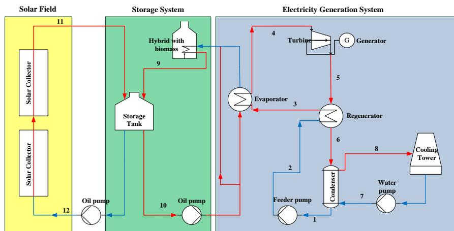
Figure 1. Schematic of Regenerative Organic Rankine Cycle (RORC)
