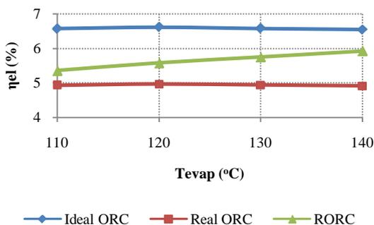
Figure 12. Electricity efficiency at varying evaporating temperature
