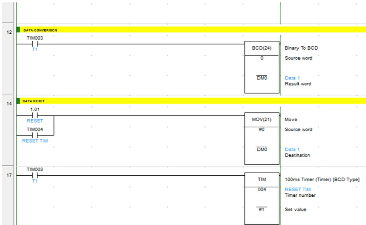
Figure 7. Ladder diagram 2 of detector input
