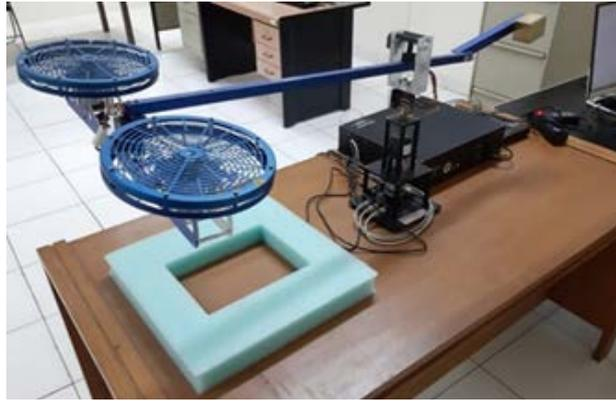
Figure 1. The experimental platform of 3 DOF helicopter as bicopter simulator
