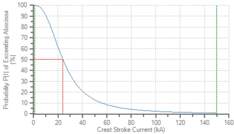
Figure 1. Probability of stroke current exceeding abscissa, 24 kA median value with 50 % exceedance probability is shown
