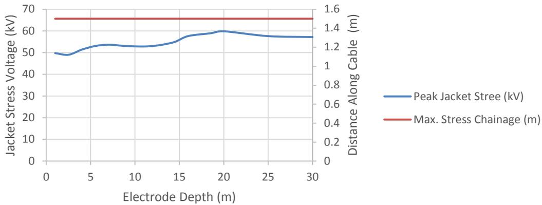
Figure 8. Peak jacket stress voltage and location variation with electrode depth
