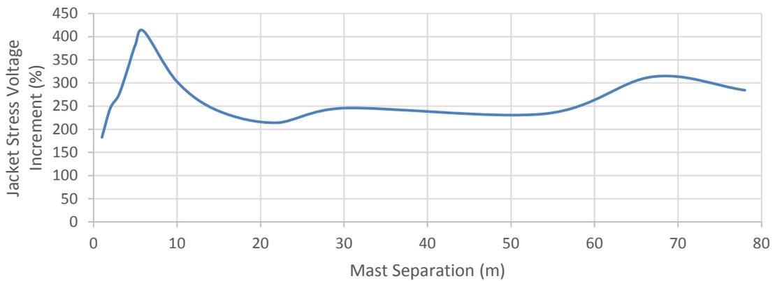
Figure 13. Peak jacket stress voltage increment with 500 Ω.m soil vs. LM separation
