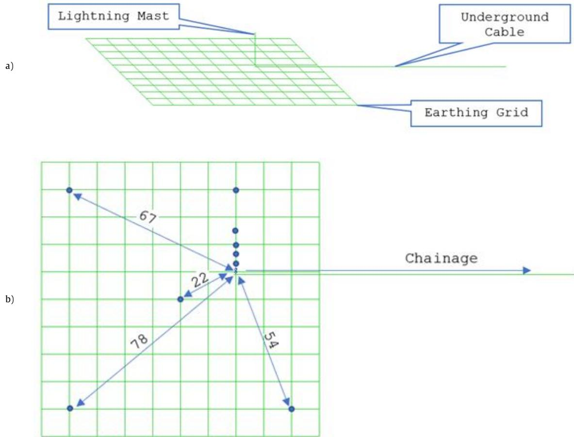
Figure 4. 100 x 100 m, 10 m uniform spacing earthing grid, underground cable, and lightning mast CDEGS HIFREQ model: (a) 3D view; (b) Plan view with LM possible locations shown in blue dots and separation distances in metres as marked. Cable chainage direction shown away from grid
