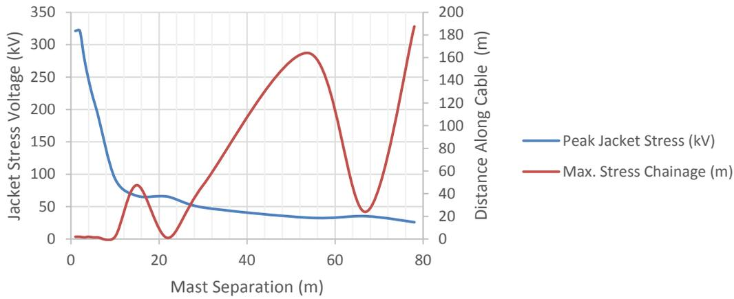
Figure 10. Peak jacket stress voltage and location variation vs. LM separation
