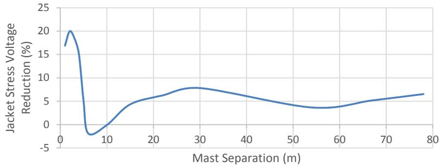
Figure 7. Peak jacket stress voltage reduction with/without electrode vs. LM separation (negative reduction % indicates stress increment with electrode)
