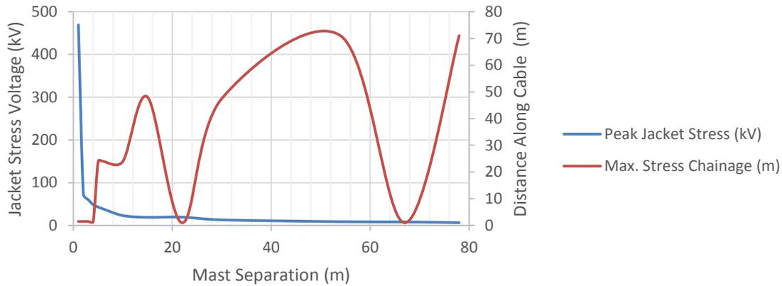
Figure 15. Peak jacket stress voltage and location variation vs. LM separation
