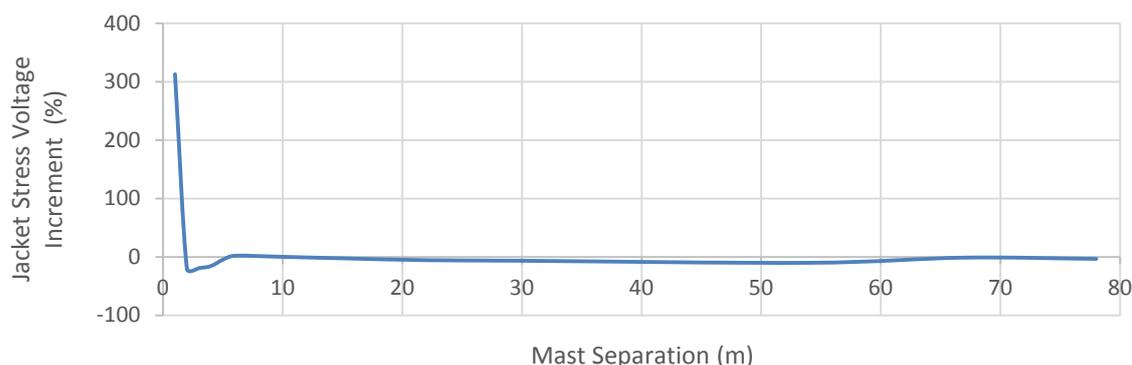
Figure 17. Peak jacket stress voltage Increment with 120/24 kA vs. LM separation (negative increment % indicates stress reduction with 120 kA lightning)
