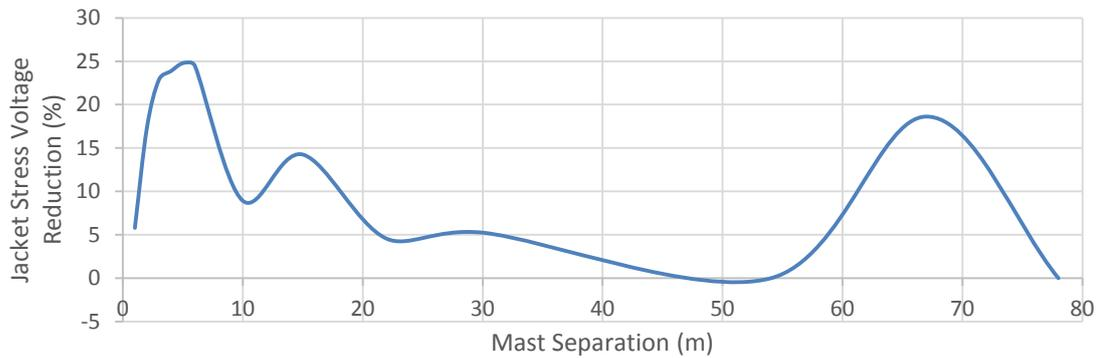
Figure 12. Peak jacket stress voltage reduction with/without electrode vs. LM separation
