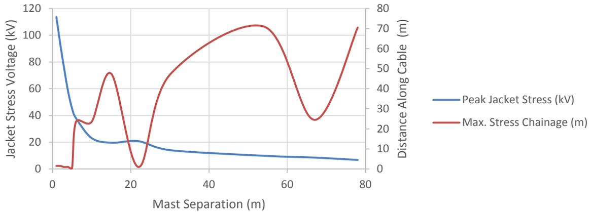
Figure 5. Peak jacket stress voltage and location variation vs. LM separation
