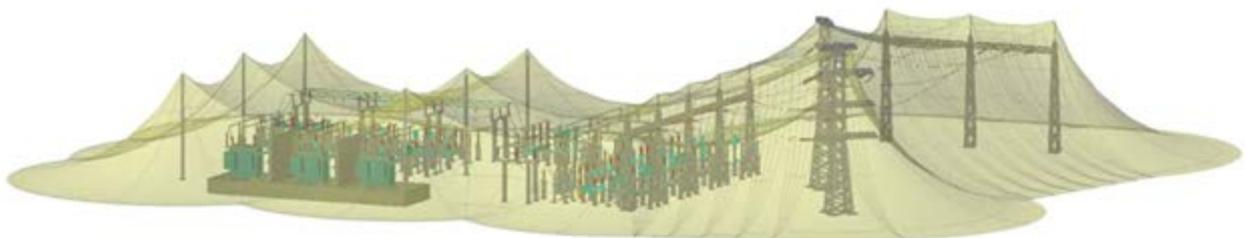
Figure 2. Lightning masts around HV switchyard and rolling sphere concept [26]
