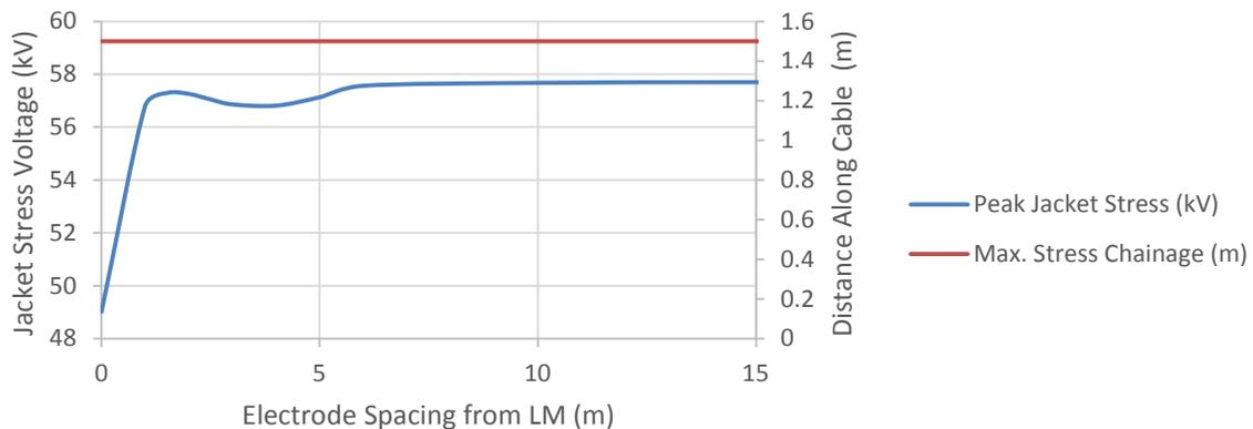
Figure 9. Peak jacket stress voltage and location variation with electrode depth
