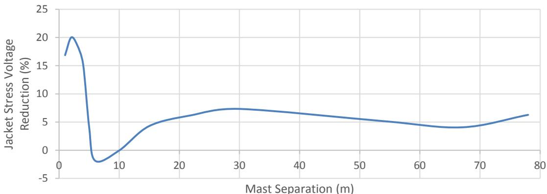
Figure 16. Peak jacket stress voltage reduction with/without electrode vs. LM separation
