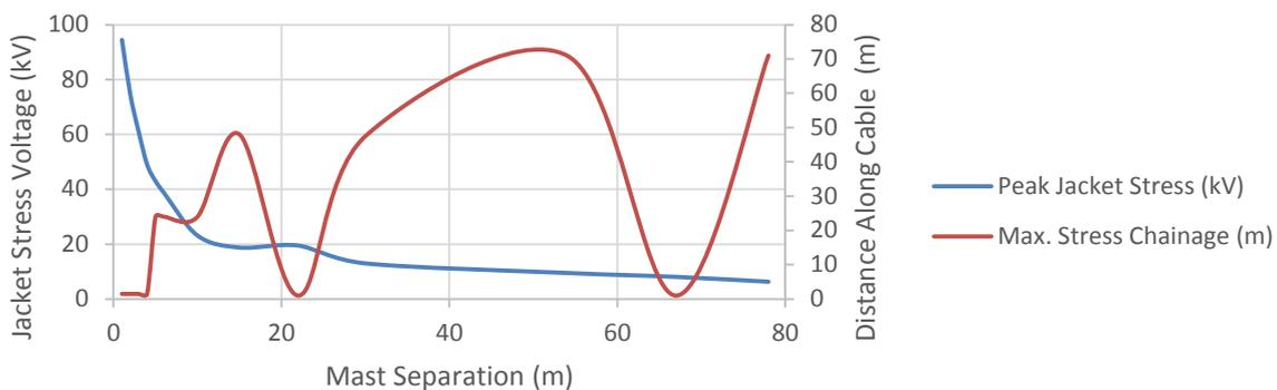
Figure 6. Peak jacket stress voltage and location variation vs. LM separation
