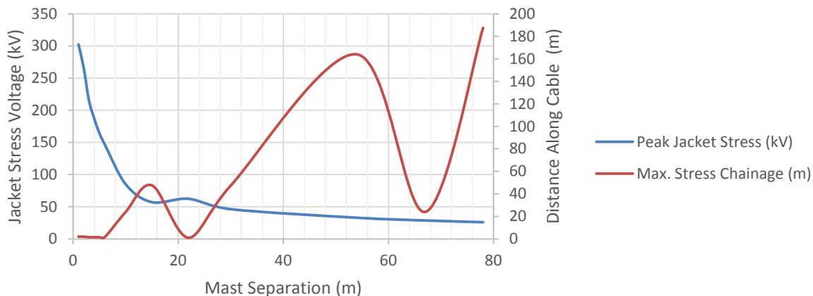
Figure 11. Peak jacket stress voltage and location variation vs. LM separation
