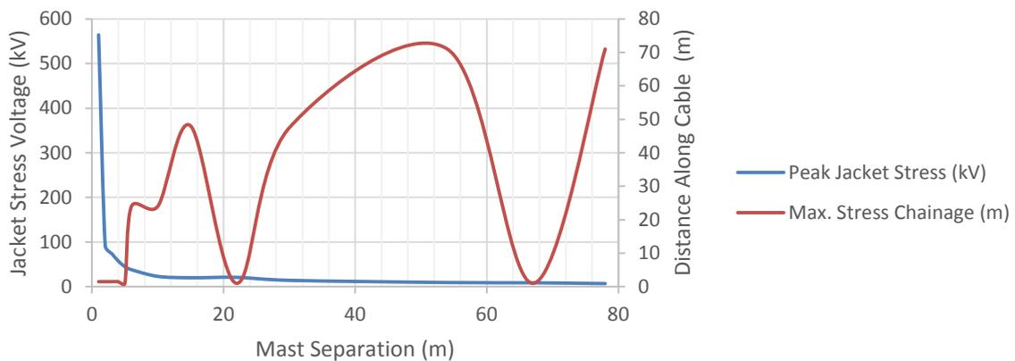
Figure 14. Peak jacket stress voltage and location variation vs. LM separation
