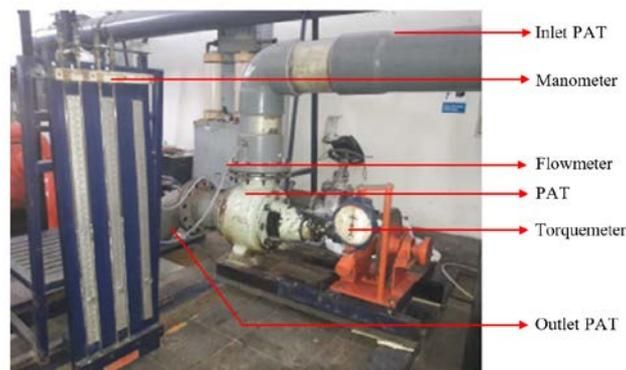
Figure 7. Assembly of PAT
