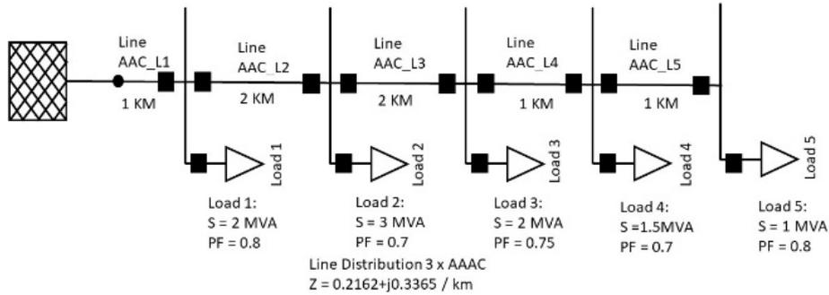
Figure 2. Radial distribution system 20 kV
