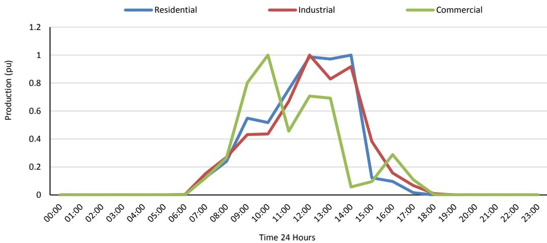
Figure 7. Photovoltaic profile characteristic
