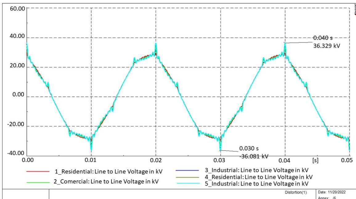
Figure 16. Voltage harmonic distortion
