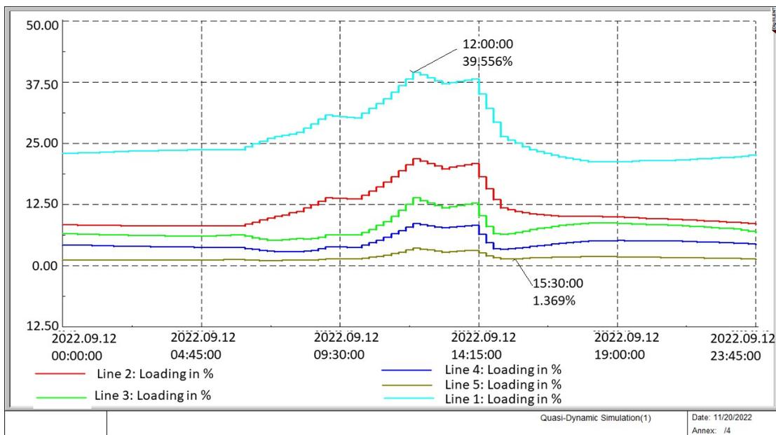
Figure 15. Thermal line loading
