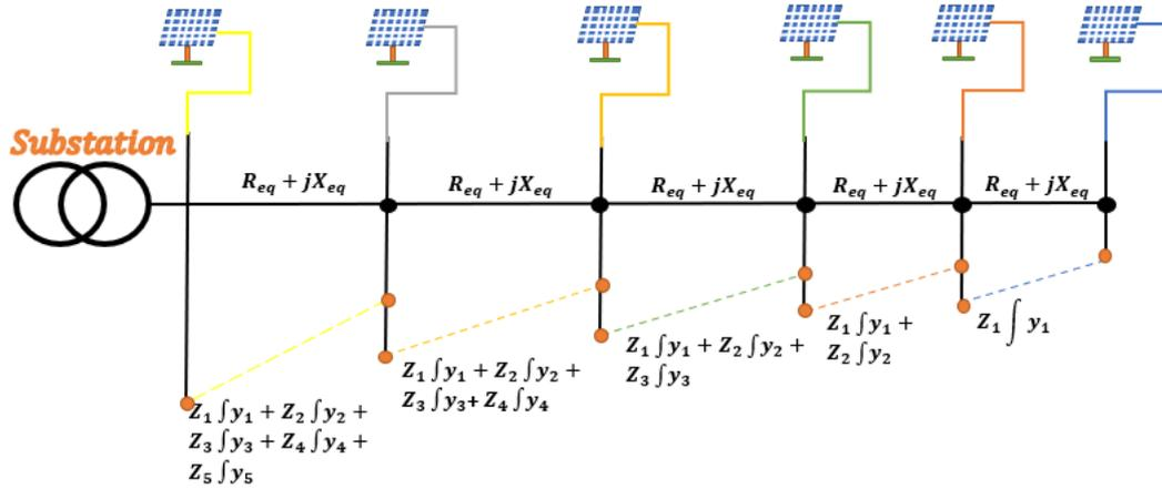
Figure 4. PV injected in each of the customers
