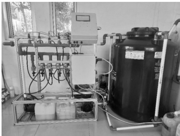
Figure 12. The nutrient dosing system prototype for hydroponic cultivation with drip irrigation.
