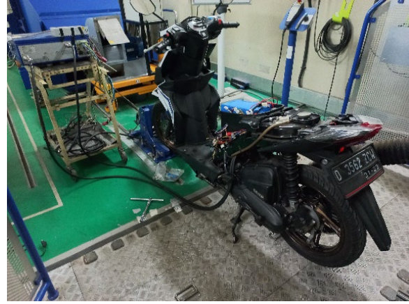
Figure 4. Modification of the fuel delivery system of motorcycles to accommodate the flow measurement.
