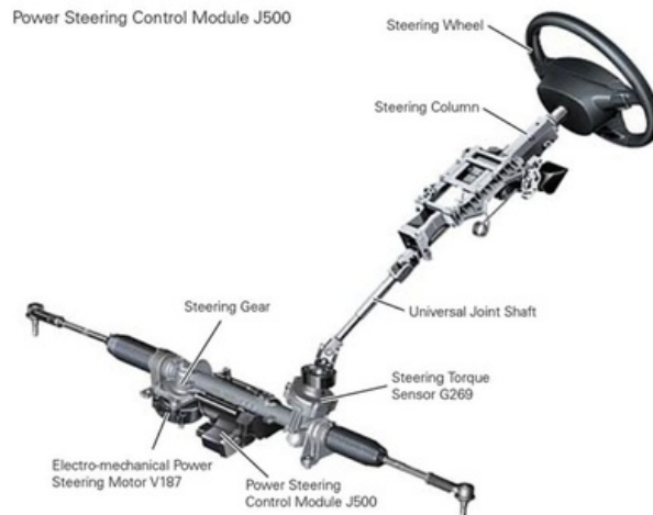
Figure 1. Steering system scheme on the main components that constitute it [2]
