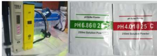
Figure 7. pH sensor calibration
