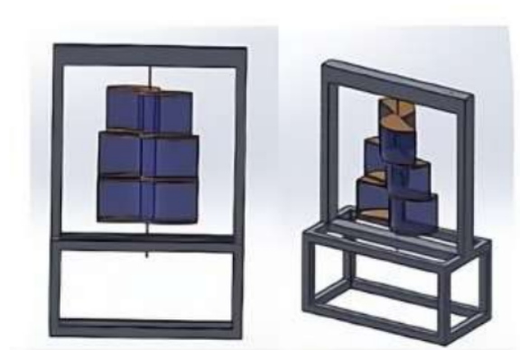
14 15 Figure 1 Multistage Savonius Wind Turbine with Fixed Rotary Axis [8]
