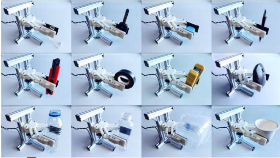
Figure 10. Grasping of objects with different shapes and sizes using the proposed gripper
