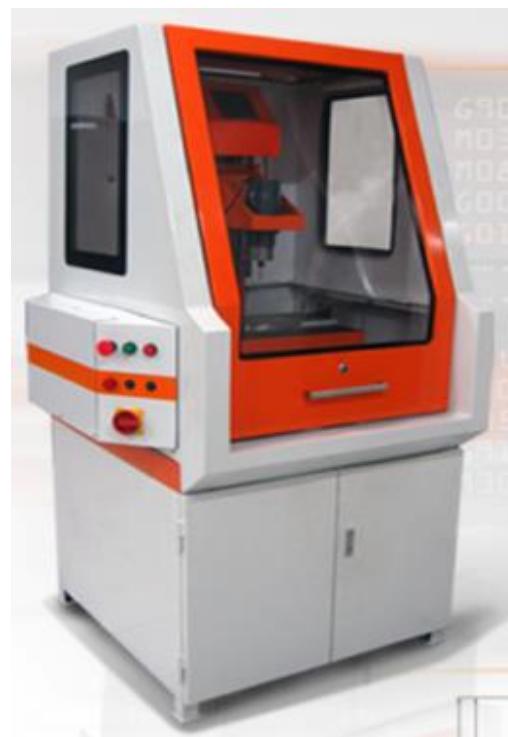
Figure 4. The prototype of 3-axis CNC milling machine developed at RCEPM-LIPI
